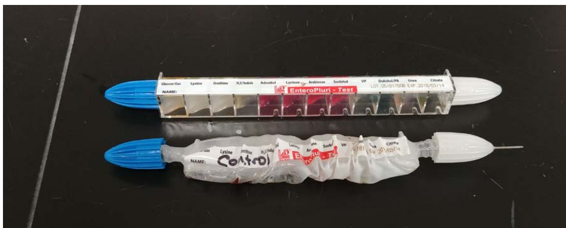
Figure 4. Un-autoclaved enterotube (top) and autoclaved enterotube (bottom). The enterotube inoculating needle protrudes from the media holder after autoclaving resulting in a sharps hazard.
